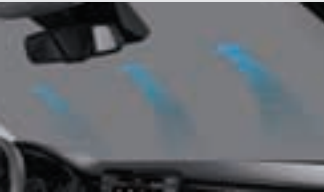
Auto defog system The auto defogger detects mist on the windshield, and automatically deploys the fans to clear the glass rapidly.
